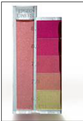
Figure F5.2: HACH Color Cube Comparator
